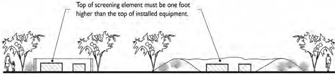
FIGURE 9311.7-B: SCREENING OF GROUND-MOUNTED EQUIPMENT
